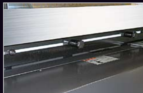
左右送り幅決め用ドグ。 Dogs for setting a longitudinal distance.
